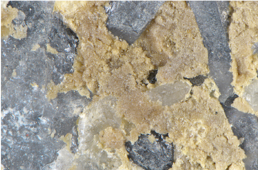
Fig. 2 Photograph of the crystalline coatings of the intermediate member of the scorodite - strengite series from Kutná Hora ore district, Czech Republic; field of view 1.7 mm.
