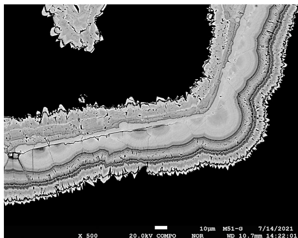
Fig. 4 Detail on chemical zoning of minerals of the hidalguito-philipsbornite series from the Guatomo mine. BSE image by T. Mikuš.
